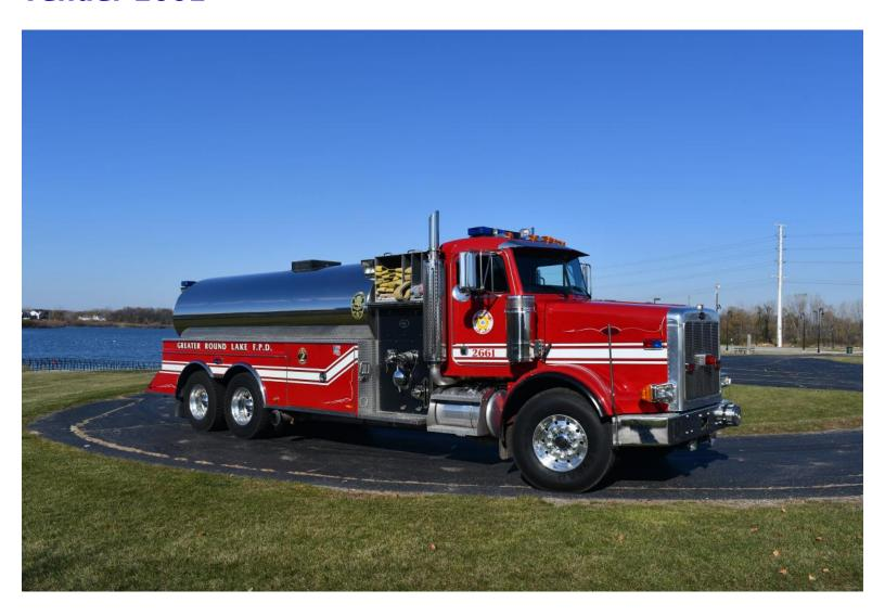
Tender 2661 is a 2000 Peterbilt tanker truck and was built by US Tanker Fire Apparatus in Delavan, WI. It carries two firefighters, has an 3,000 gallon water tank and can pump 1,250 gallons per minute. It also carries a 2,500 gallon portable water tank and has a rapid dump valve on the rear of the tank for water shuttle operations. Tender 2661 has responded to incidents of national significance including deployment to Louisiana for Hurricanes Gustav and Ike in 2008.
