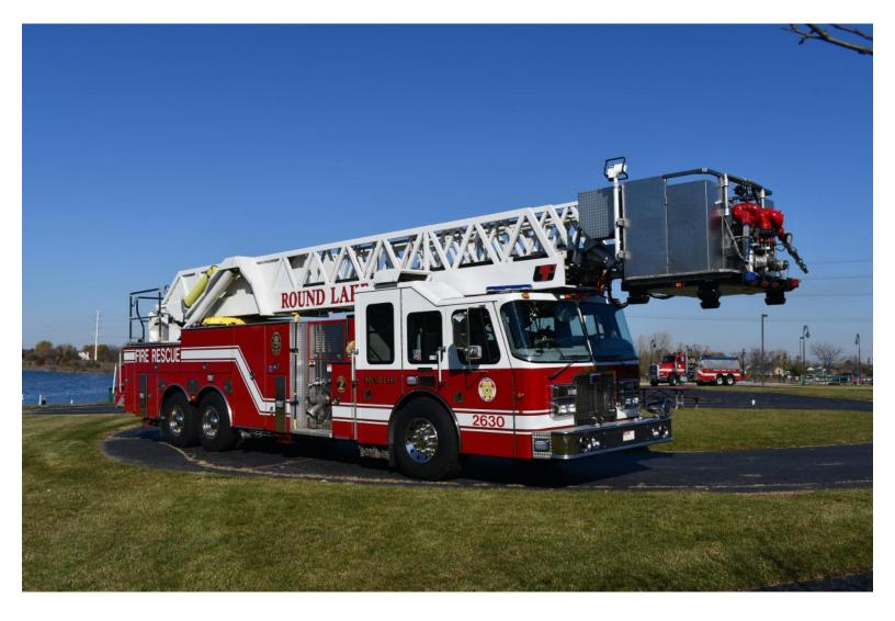
Ladder Tower 2630 is a 1998 Simon Duplex ladder truck and was built by Ladder Towers Incorporated (LTI) in Ephrata, PA. It carries four firefighters, has an 250 gallon water tank and can pump 2,000 gallons per minute. The main ladder is 102' long and has two master stream nozzles attached to the basket. Ladder Tower 2630 has responded to incidents of local and national significance including the 2004 LaSalle Bank fire in Chicago and to New Orleans in 2005 for Hurricane Katrina.
