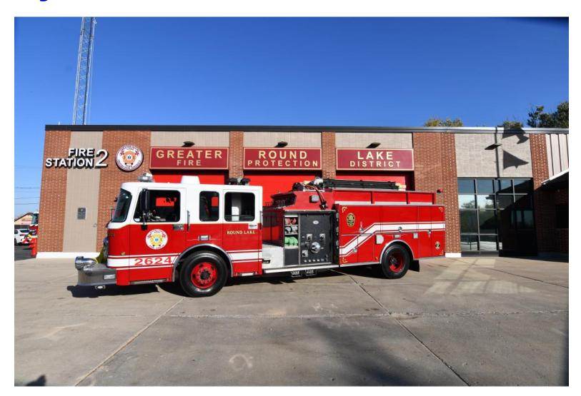
Engine 2624 is a 2004 Spartan chassis and was built by US Tanker Fire Apparatus in Delavan, WI. It carries four firefighters, has an 800 gallon water tank and can pump 1,250 gallons per minute.
