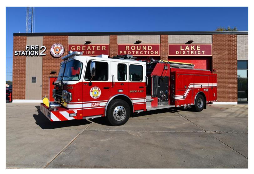
Engine 2622 is a 2019 Spartan chassis and was built by Custom Fab & Body in Marion, WI. It carries four firefighters, has an 800 gallon water tank and can pump 1,250 gallons per minute.
